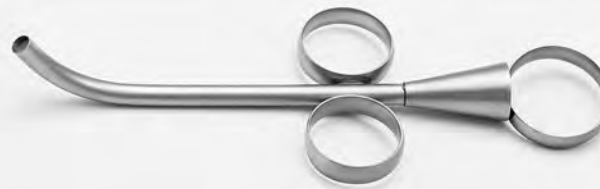
Ridge mapping caliper, For Mapping Bone Width 0-25 mm range
